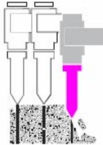
Use a gradual approach to breaking up material section by section. Start at the edge of large pieces, then work in towards center.
