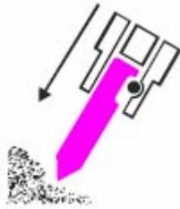
The correct strike position should be a 90° angle to the work surface. The shank, chuck and carrier should form a unit.
