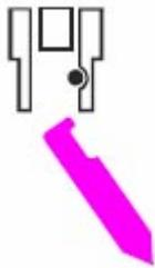
Apply grease on high-stress tools especially liberally before inserting into the hammer.
